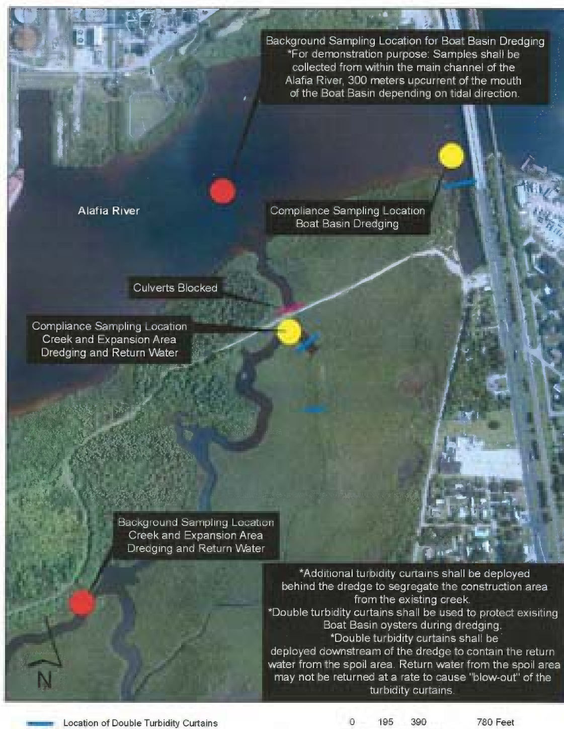
Figure 1. Turbidity monitoring locations and turbidity curtain locations for the Return Water Discharge, Boat Basin Dredge, and Creek Dredge.
