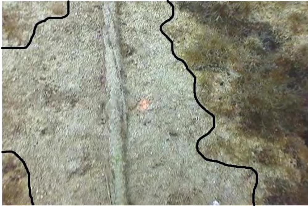
**Figure 15.** An example image grabbed from a transect video of cable scour from site IR1-C. The outlined scoured substrate and the worn cable provide evidence of cable movement.
