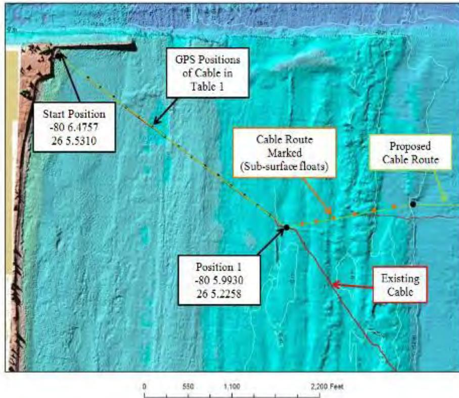
Figure 9: Diver Survey of Gateway Cable
