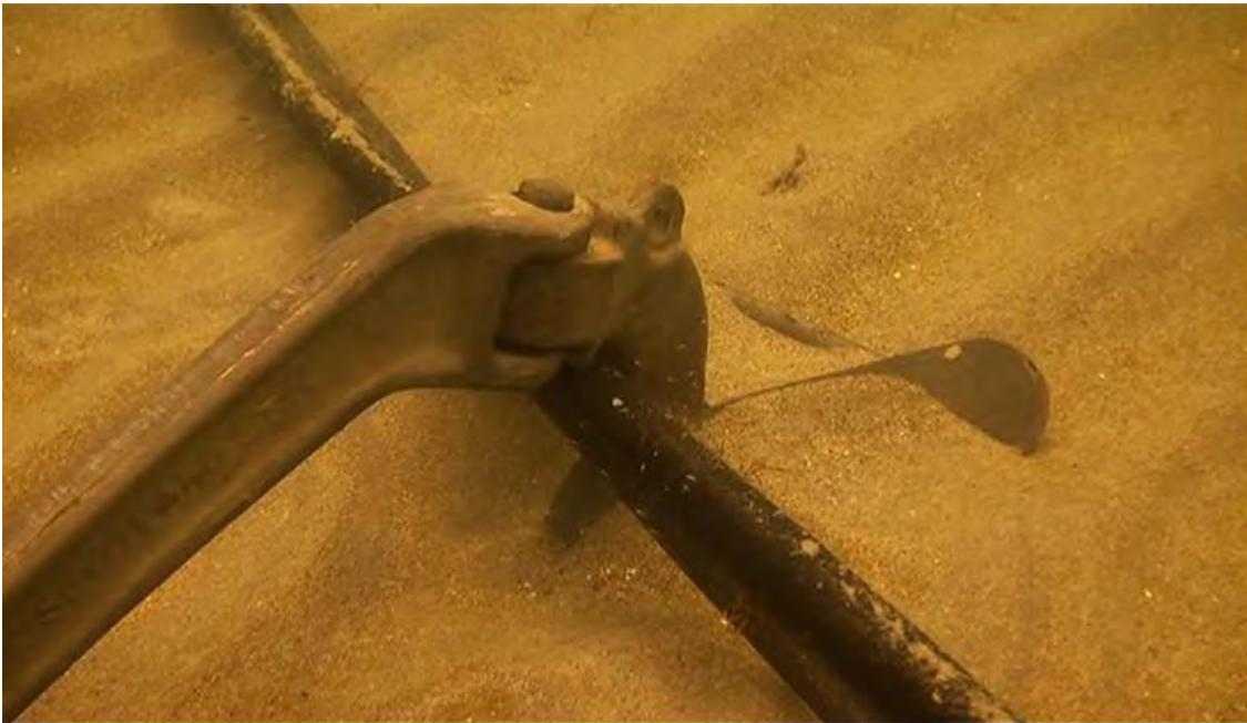
Figure 10: Example of boat anchor entangled in sea cable.
