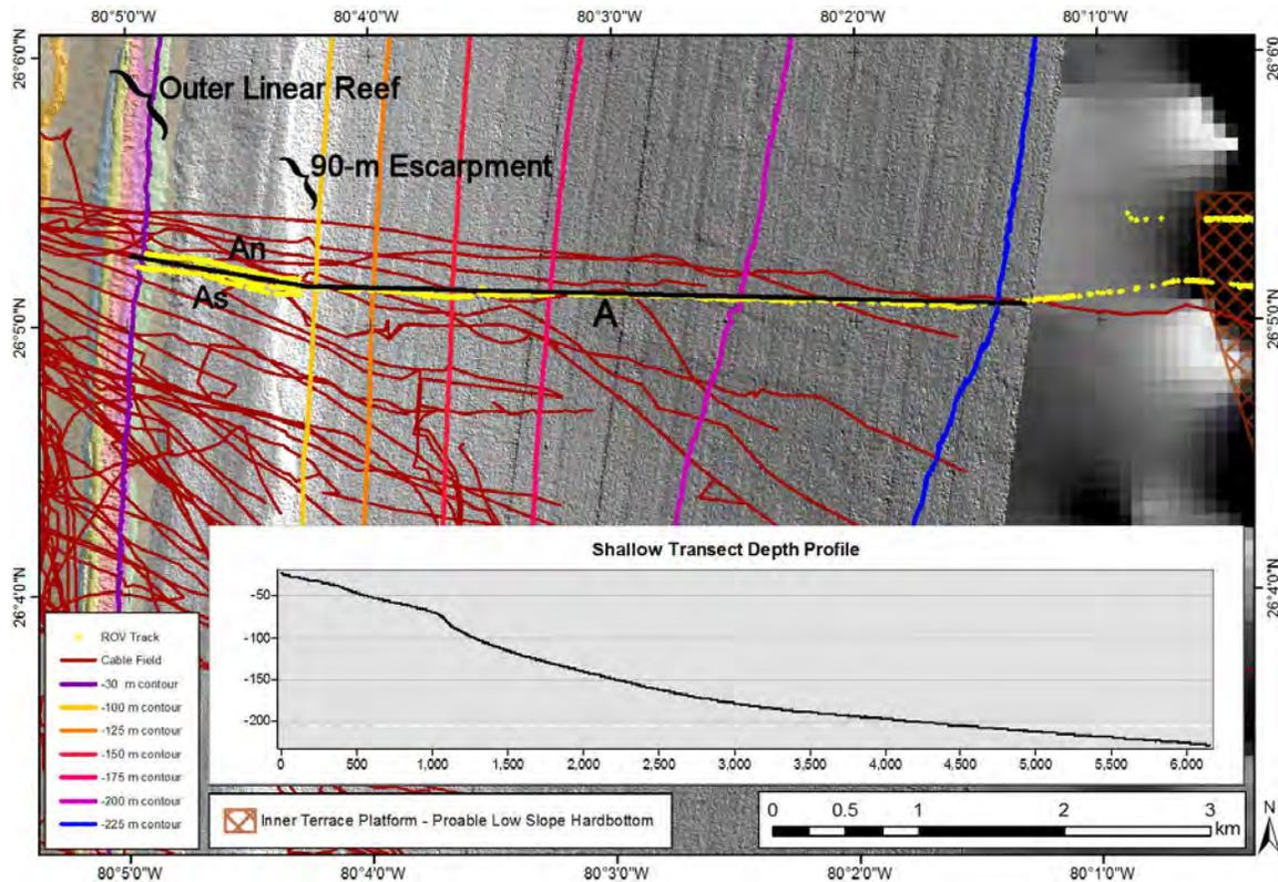
Figure 4-4. ROV Cable transect (transsect A as in Figure 4-1) from western terminus in ~30 m to ~230 m (yellow line) with corresponding depth profile (black line) to just over 225 m shown in insert. The shallow (~30-90 m) North and South parallel Non-Cable transects (As and An) are visible at left. Background bathymetry: 2001 US Navy multibeam bathymetry.
