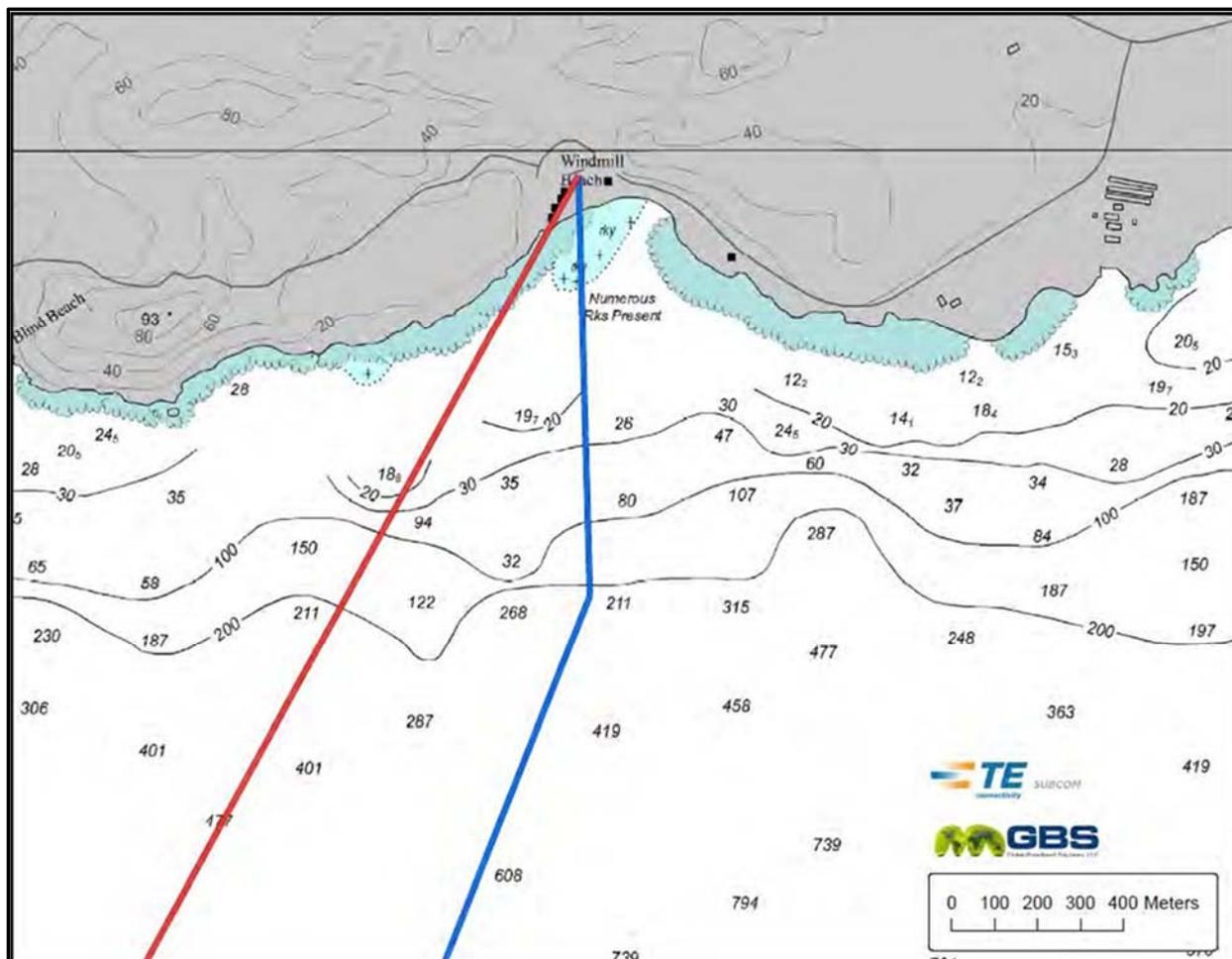
Figure 16 Alternative nearshore approaches to Windmill Beach
