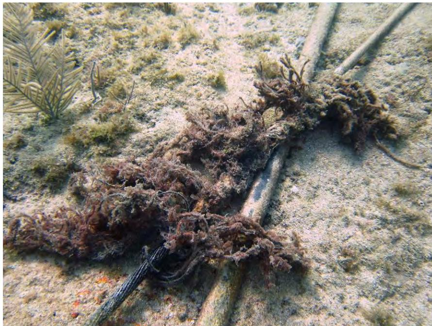
**Figure 21.** An example of a frayed cable in the CPS habitat. Movement of the smaller diameter cable along the larger cable is also evident.
