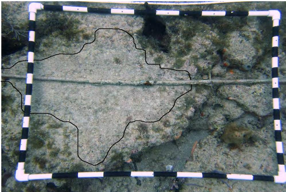
**Figure 16.** An example of a quadrat (75x100 cm) with scour from the site IR1-C belt transect. The outlined scoured substrate and the worn cable provide evidence of cable movement.
