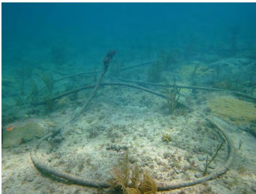
**Figure 20.** An example of a broken cable in the CPS habitat. The broken end and the non-linear position of the cable provide evidence of cable movement.
