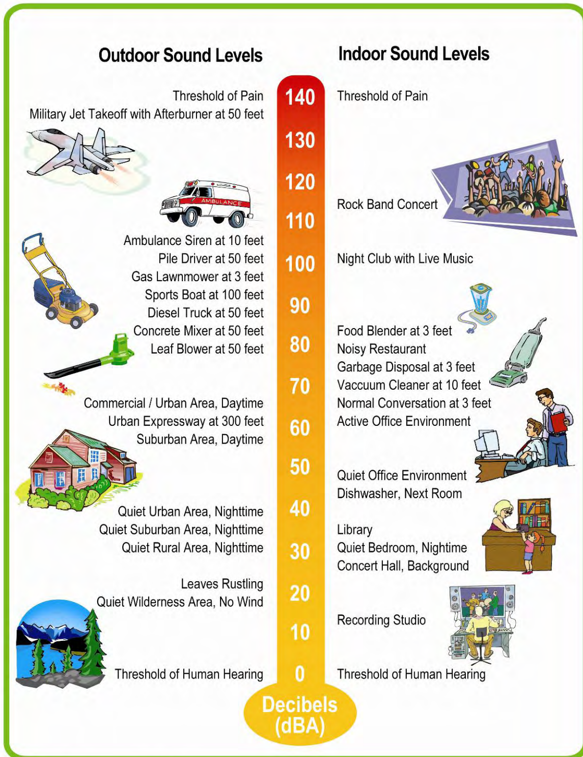
Figure 1. Sound Levels of Typical Noise Sources and Noise Environments
